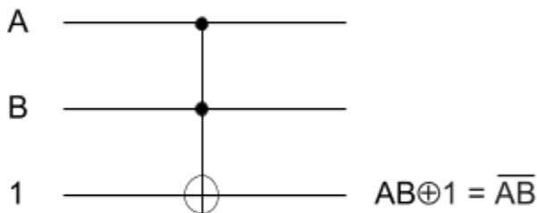
The third bit ends up as 0 if only if both A and B are both 1, meaning that the third bit gets flipped. Thus, we've got a NAND gate.
