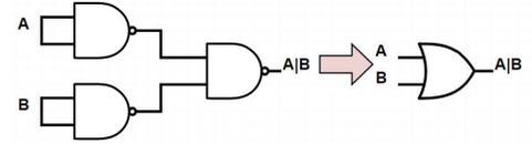
By contrast, the set {AND,OR} is *not* universal, because it can only express monotone Boolean functions: that is, changing an input bit from 0 to 1 can never change an output bit from 1 to 0. Likewise, the set {NOT,XOR} is not universal, because it can only express Boolean functions that are linear or affine mod 2. So, while “most” gate sets are universal, being universal isn't completely automatic.
